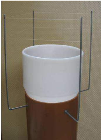
Figure 11: The end look of the bird ring with the funnel in place.
