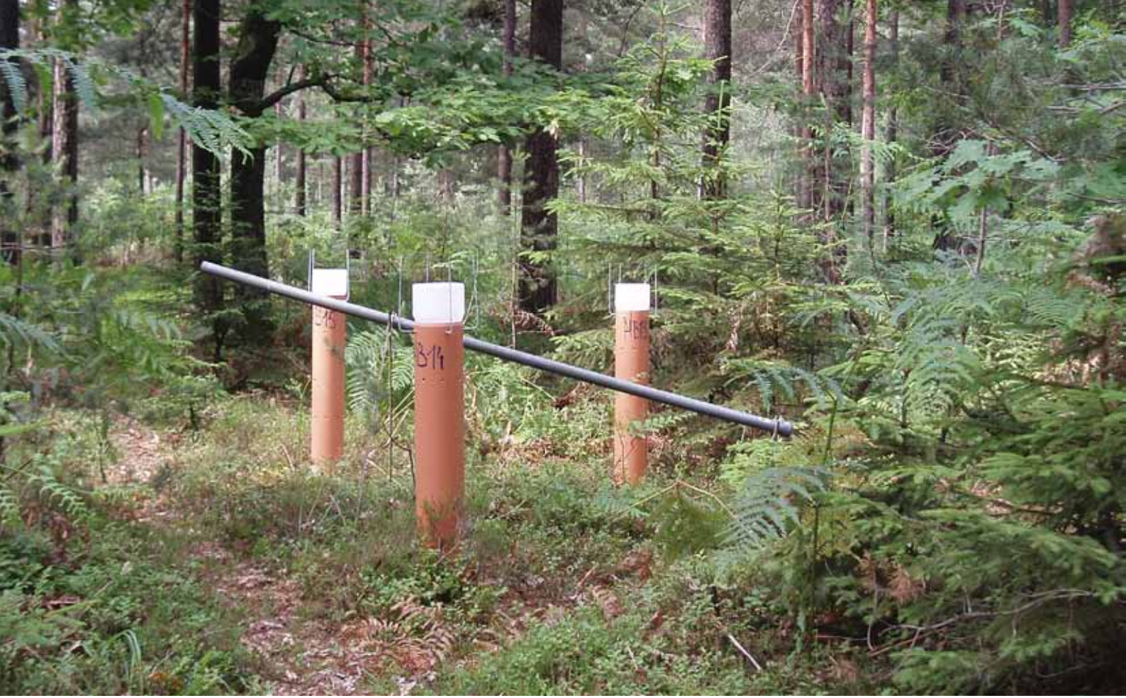
Nutrient cycles in the forest: Different types of deposition samplers are being tested in Slovenia.
