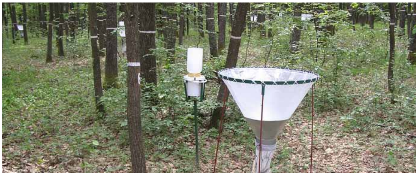
Litterfall and deposition sampler on an intensive monitoring plot in the Slovak Republic
