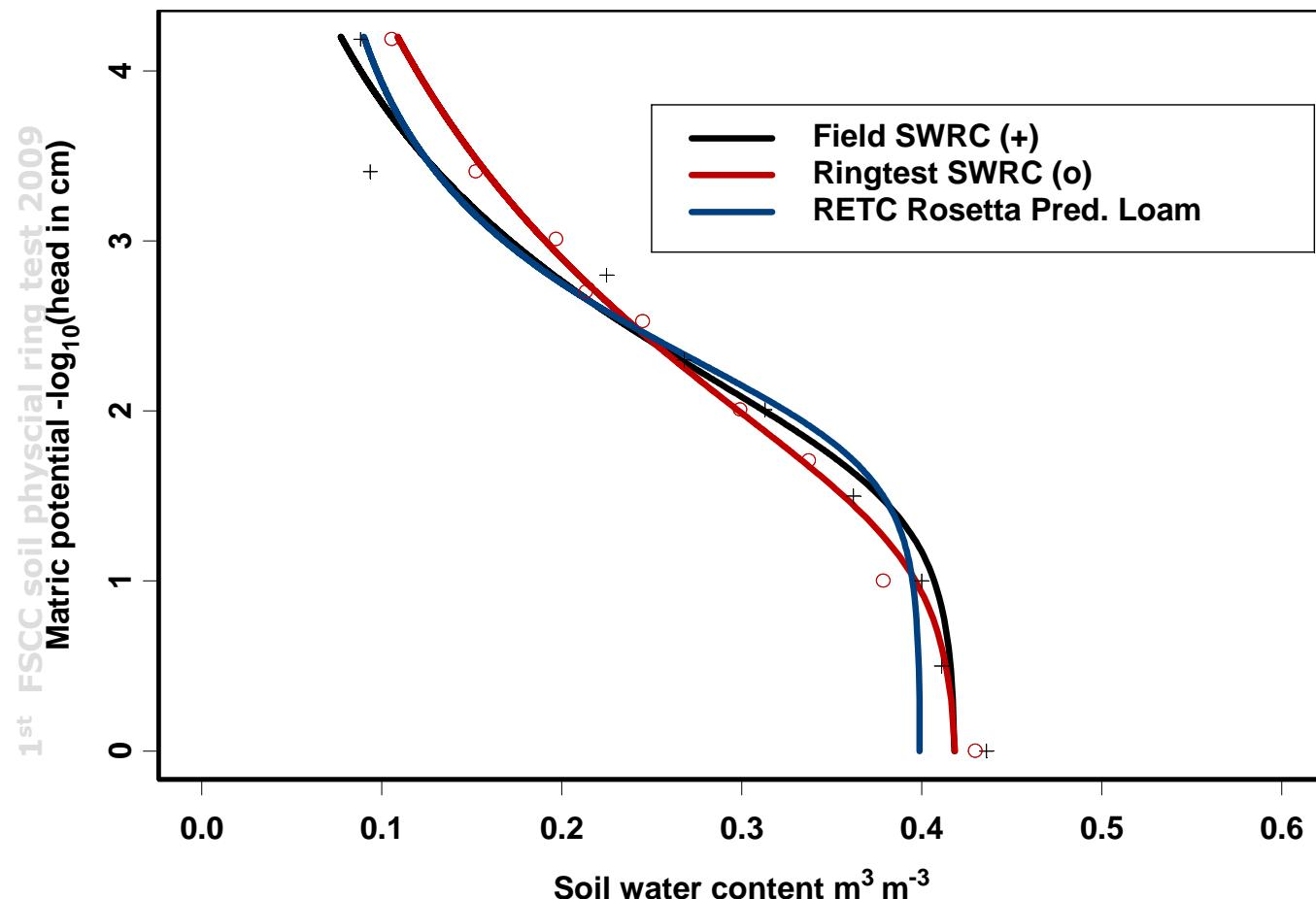
Neural network prediction based on texture class is close to VG fitted SWRCs (some deviance for low pressures)
