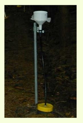
We should cool samples – Sampler in soil pit is a solution, but:
